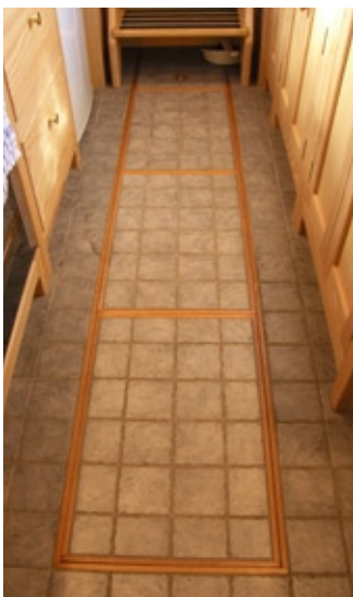
Multiple cabin bilge access hatches in the tiled galley floor, plus access to bilge pump for cabin.
